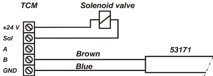
The TCM port should be set to control the appropriate PC tank in relation to the physical tank. Correct TankType, TCMAddress and TCMPort should be set using with WinDB Manager.
