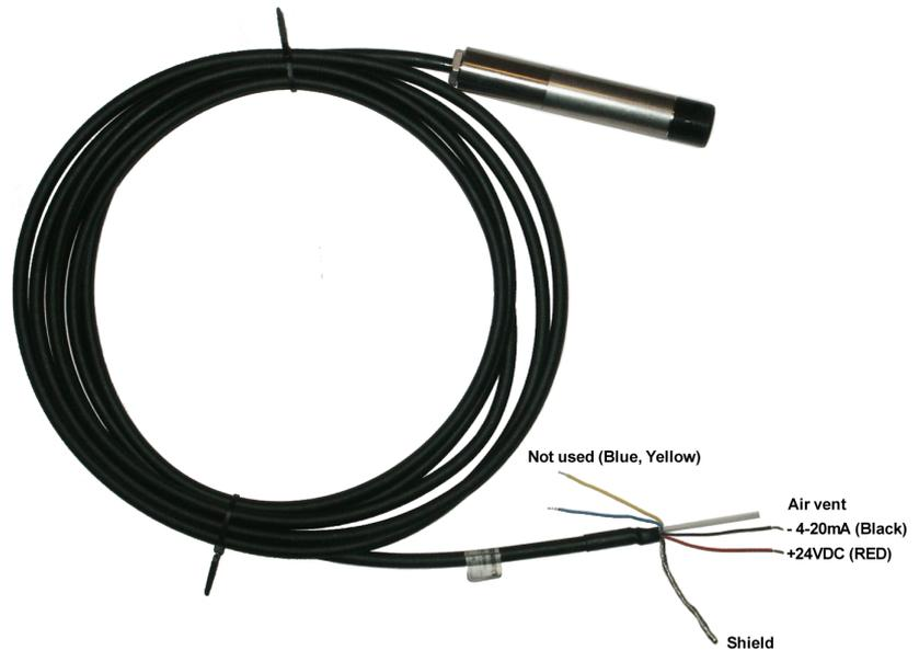
It is not necessary to use the shield to obtain a good signal because the signal is current based. The shield can be used for protection grounding purposes if needed.
