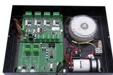
Fasten the short plastic distances so the new card can be placed closest to the bottom like in the picture. The printer module cable is then easily installed in the correct position.
