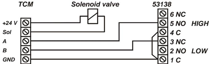
The TCM port should be set to control the appropriate PC tank in relation to the physical tank. Correct TankType, TCMAddress and TCMPort should be set using with WinDB Manager.
