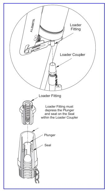
**Figure 6** Loader Fitting and Loader Coupler Section View
