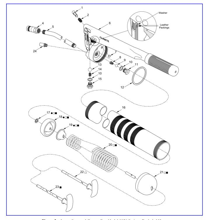
Figure 2 Lever-Operated Grease Gun Model 1056 Series - Exploded View
