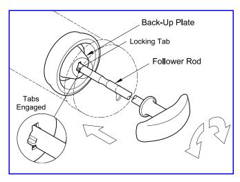
Figure 5 Follower Rod Engaged with Back-Up Plate
