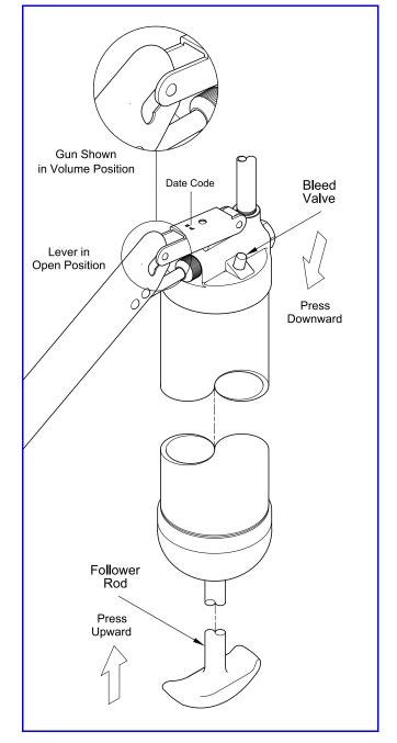
Figure 7 Force Priming the Gun
