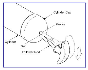
Figure 3 Follower Rod Engaged in Cylinder Cap Slot
