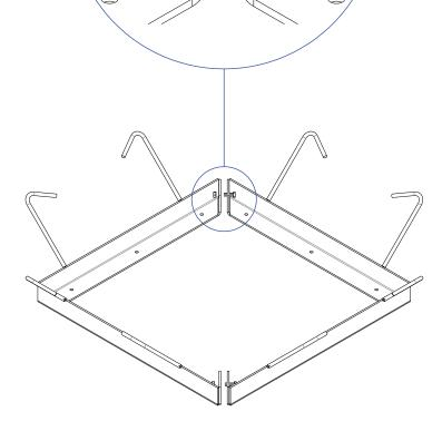
Minimum 800 mm in order for the bolts to clear. It can be more than 800mm but then it will be less surface area to carry the weight.
